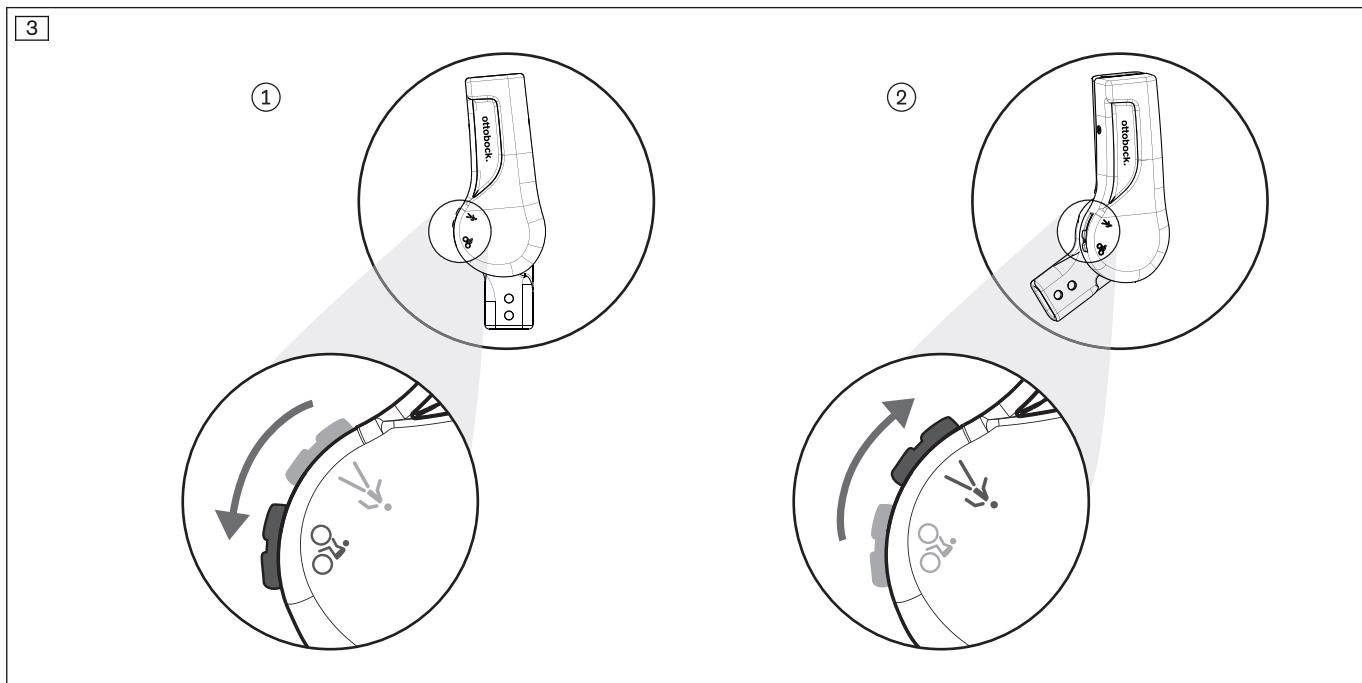
For certain activities (e.g. cycling), it may be beneficial to temporarily unlock the E-MAG Active joint. Mechanical unlocking of the system is indicated by the symbol of a cyclist (switch to "🚴").
