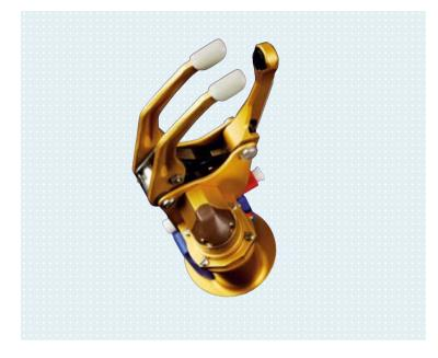
Two independent measurement and control systems proportionally control the gripping speed and gripping force. A strain gauge between the thumb and index finger recognizes whether the gripping force or gripping speed needs to be proportionally controlled.
