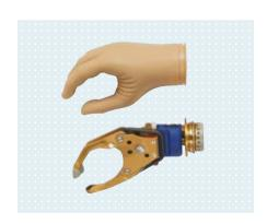
8E38=8 SensorHand Speed with Quick-Disconnect Wrist
