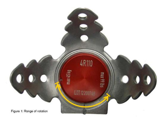
The threaded insert is **not designed to be removed** from the three prong adapter. This component has a security punch designed to limit internal or external rotation up to 45 degrees. The lamination protection cap has been provided and covers the red threaded insert during lamination.
