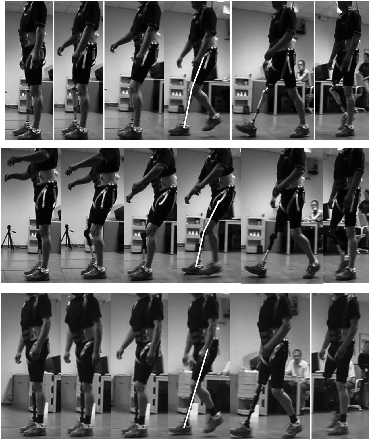
Figure 4. Phases in right-to-left chronological sequence when stopping abruptly with the three tested knees: C-Leg (top), 3R80 (middle), and 3C1 (bottom) at the instant of the hand signal (far right), heel strike of the prosthetic foot (second right), heel strike of the contralateral foot (fourth panel), and static stance (far left). During deceleration the different prosthetic knee angles are indicated in third panel.
